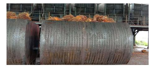
These loaded containers are subjected to sterilization (moist heat) at 5kg pressure. This is done to decontaminate the palm fruits and loosen them as steam passes into them, so that it could be easy to separate the seed from the fruit. Here they use the mesocarp of the fruit is used for the production of oil not the seed.
